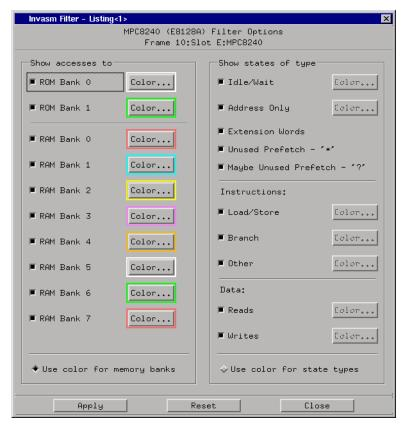
The inverse assembler filtering options allow you to display or hide certain types of microprocessor bus cycles or memory bank accesses.
