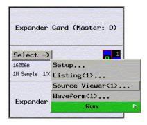
The source correlation tool set correlates the logic analyzer's address label with a line of high-level source code whose address, symbol name, file name, and line numbers are described in a symbol file downloaded to the logic analyzer (see "To load object file symbols" on page 111).
