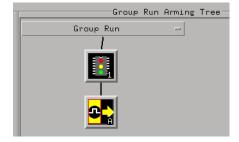
Selecting the **Group Run** button (at the very top of the Intermodule window or a logic analyzer window) will start the analyzer running. The analyzer will
