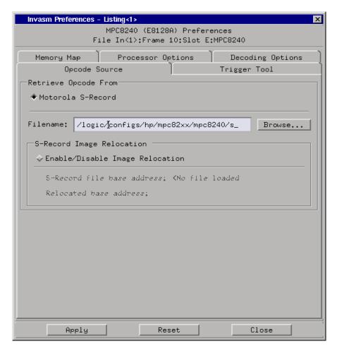
**Specifying use of Motorola S-record executable file.** Select **Motorola S-Record** in the **Retrieve Opcode From** dialog to have a Motorola S-record supply execution trace information to the cache-on trace reconstruction tool. Use the **Browse...** button to locate the S-record file.
