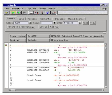
The inverse assembler is already loaded when state configuration files are loaded, but it can also be loaded into a Listing display using the Invasm menu. The name of the inverse assembler file is I8620E, and it is located in the /logic/ia directory.
