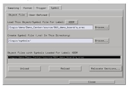
When you load object file symbols into a logic analyzer, a database of symbol/line number to address assignments is generated from the object file.
