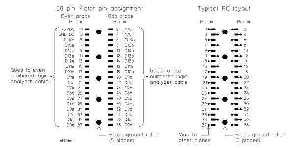
Five center inline pins on the connector are the signal ground returns and must be connected to ground.
